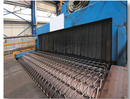
Work piece exit with blow-off ventilator
