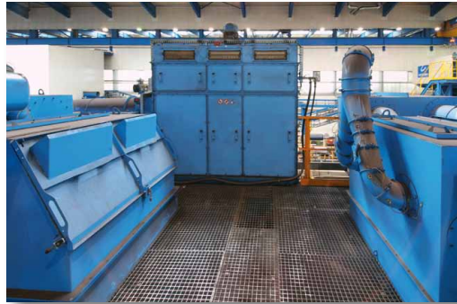
Cartridge filter system and cascade wind sifter for removal of dust and undersized particles from the abrasive
