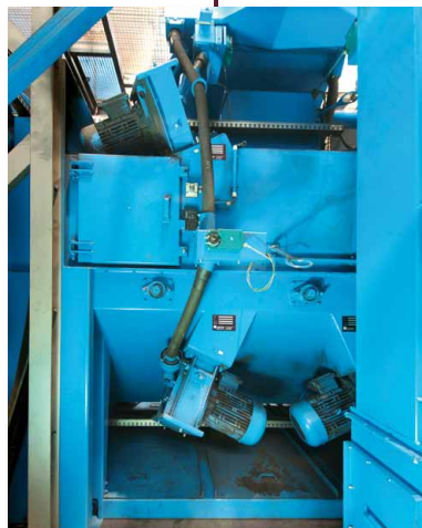
Blasting chamber with AGTOS high-performance turbines
