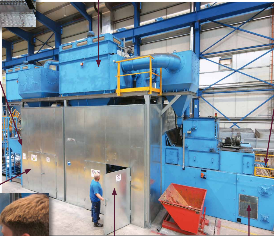
Cartridge filter system and cascade wind sifter for removal of dust and undersized particles from the abrasive
